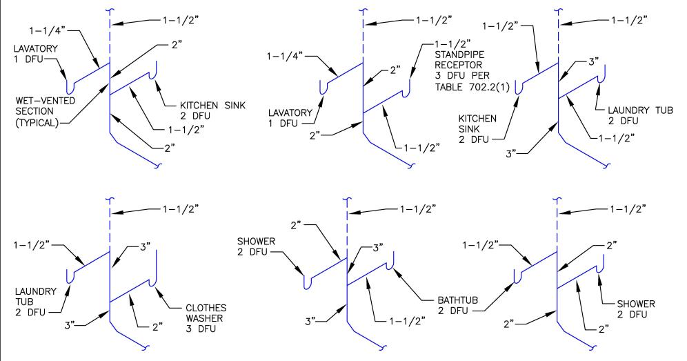
NOTE: ALL FIXTURES SHOWN ARE PRIVATE USE, ALL PIPE SIZES SHOWN ARE MINIMUM PIPE SIZES REQUIRED, AND NOT ALL REQUIRED CLEANOUTS ARE SHOWN
