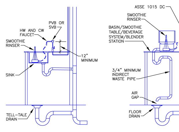
DC = DOUBLE CHECK VALVE BACKFLOW PREVENTION ASSEMBLY
