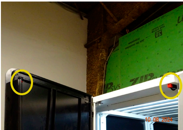
The Bodor Laser CNC main access door with a properly installed tongue-style interlock switch (upper left-hand corner).
