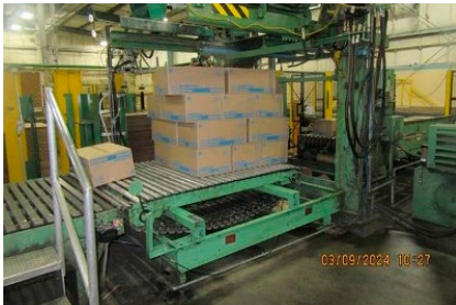
Georgia Pacific's stacking machine with the guards removed.
