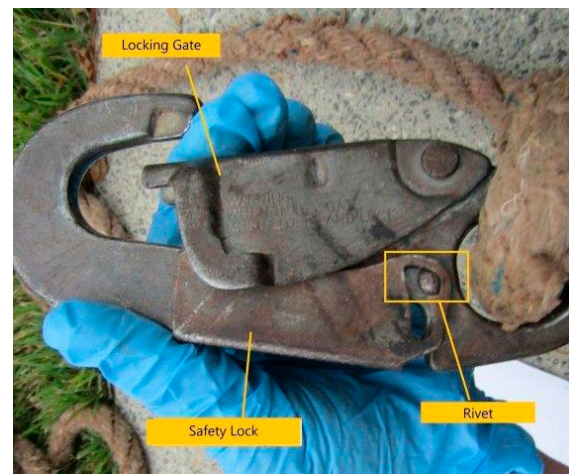
Locking clasp on rope grab.
