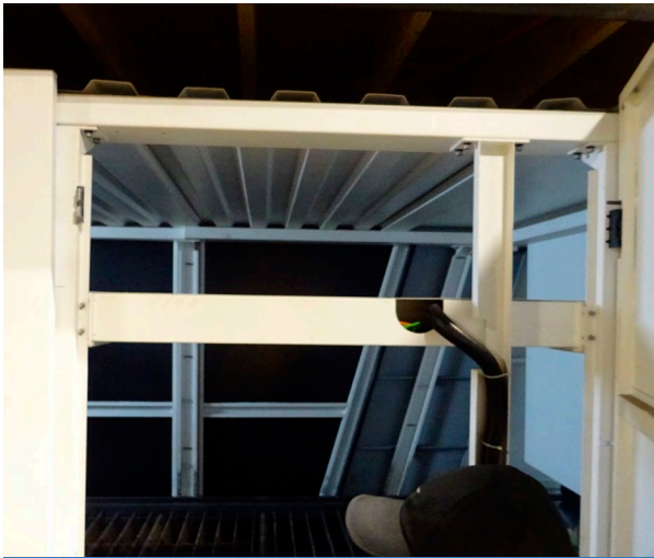
One of the Bodor Laser CNC side maintenance doors, where the accident occurred, with no safety door switch installed.
