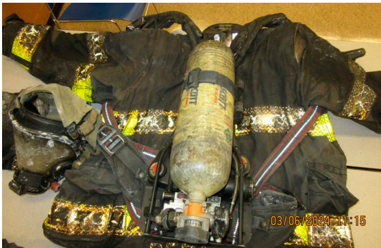
Turnout gear worn by firefighter who sustained burns while fighting a structural fire.
