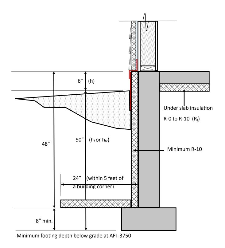
Semi-heated Garage Foundation Section Diagram
