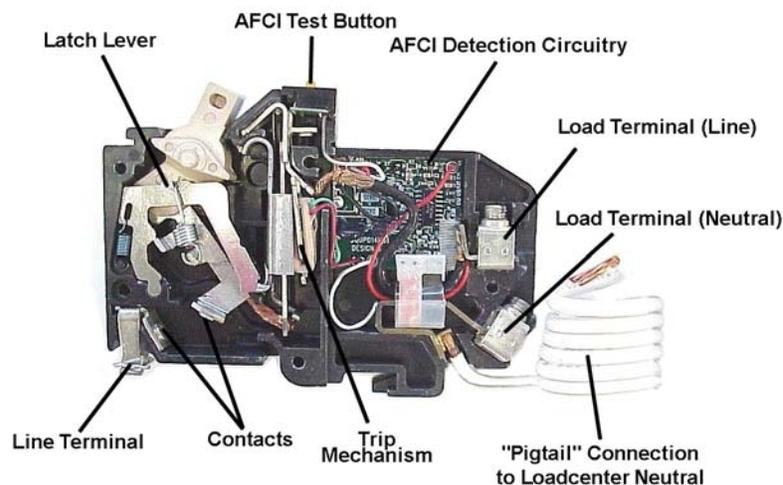
Fig. 16 – Modern AFCI Circuit Breaker
