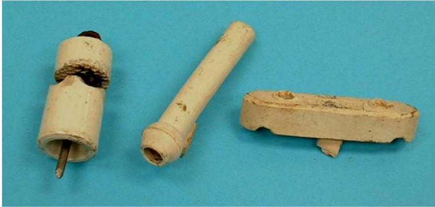
Fig. 2 – Old Knob, Tube, and Cleat
