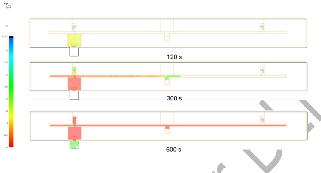
Figure H6. FDS visibility results of the fire floor in the 40,625 sf building with stairway door open on fire floor. (Visibility tenability criterion: 15 feet)
