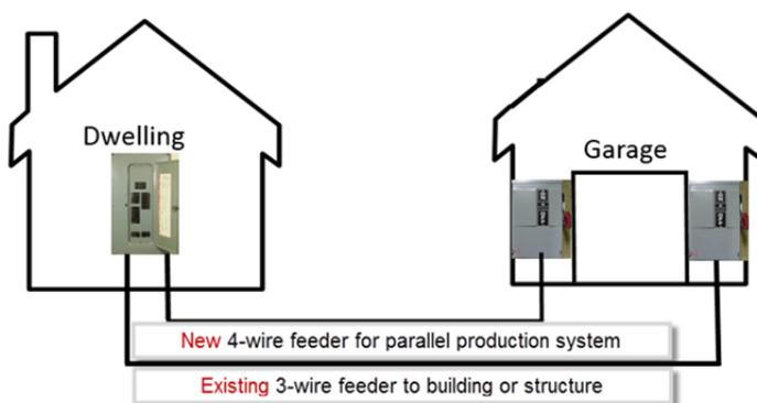
To ensure that neutral current is not continuously flowing on the new 4-wire feeder EGC, a new EGC would be required to be installed with the existing 3-wire feeder conductors, and installed according to NEC 300.3(B). The new EGC routed with the existing 3-wire feeder would be sized based on the overcurrent protection on the supply side of the feeder, according to NEC table 250.122. The equipment grounding conductors and neutral conductors would need to be separated
