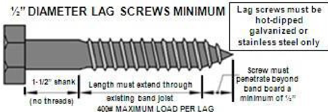
FIGURE R507.9.1.3(1) PLACEMENT OF LAG SCREWS AND BOLTS IN LEDGERS
