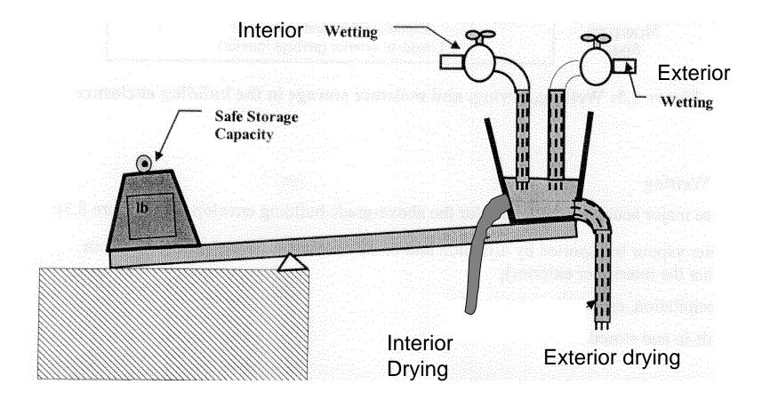
A typical house can have 10,000 pounds of studs and sheathing 10% moisture is 1,000 pounds or 125 gallons of water capacity
