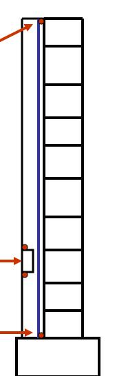
Waterproofing **shall** be applied to the entire inside surface of the foundation wall
